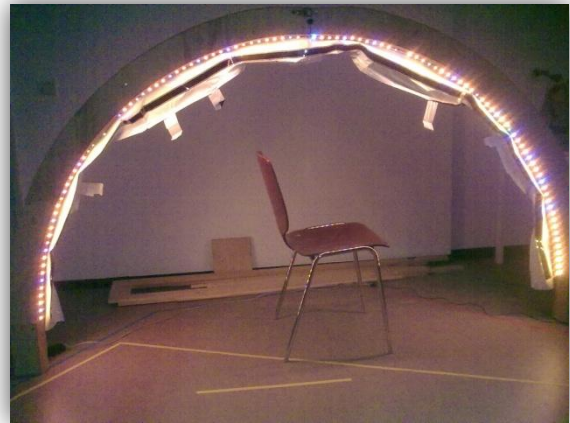
Figure 12: LED half circle with 111 individually controllable LEDs. The bed was placed where the chair stands. Stimulus intensity was controlled by the number of LEDs turned on, their color and their brightness.
